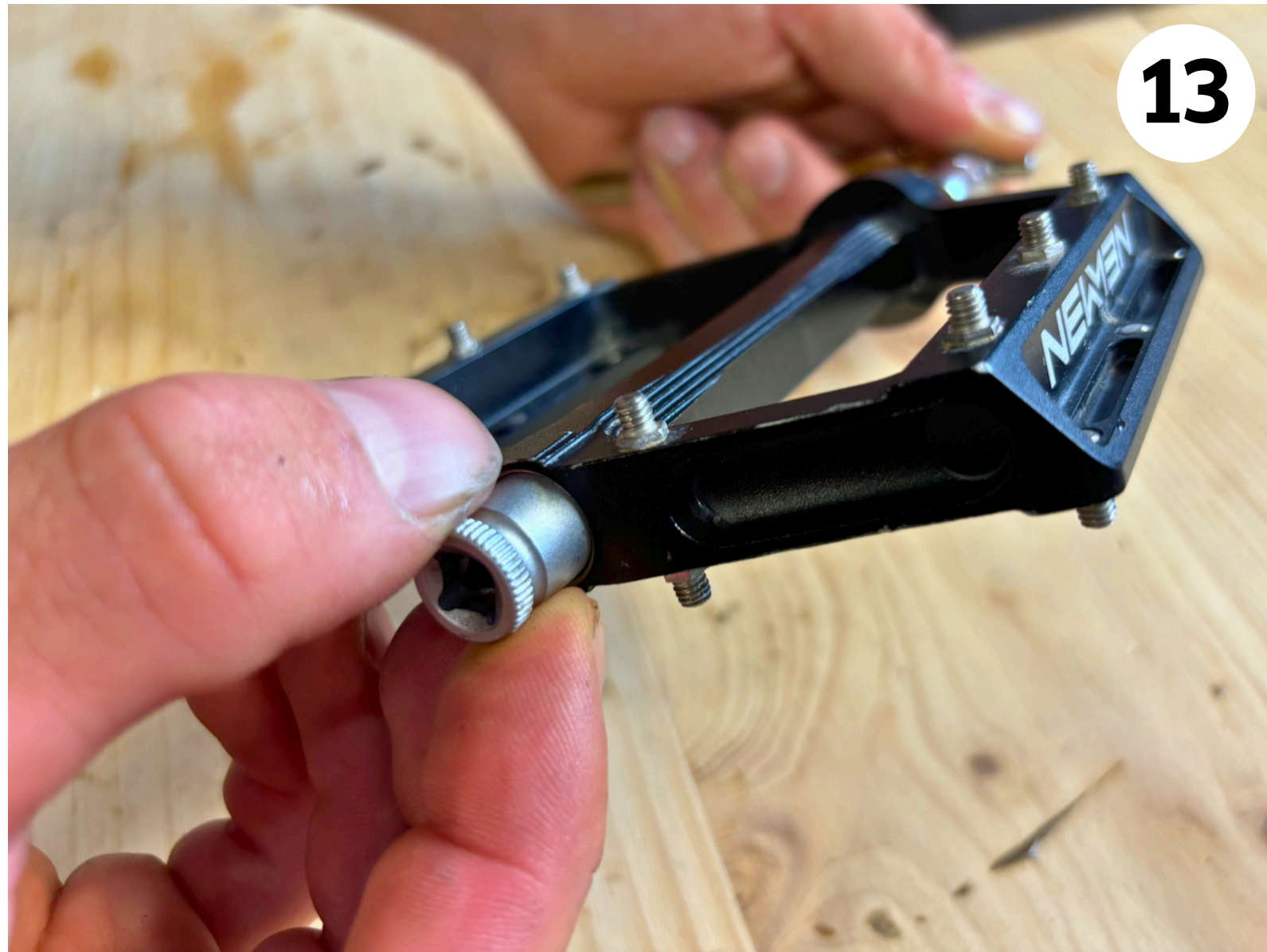
Tighten the M4 nut on the outside of the pedal by hand (!) while holding inside with a 6mm hex key. Note: The nut for the left-hand side has a right-hand thread, the nut for the right-hand side has a left-hand thread.
