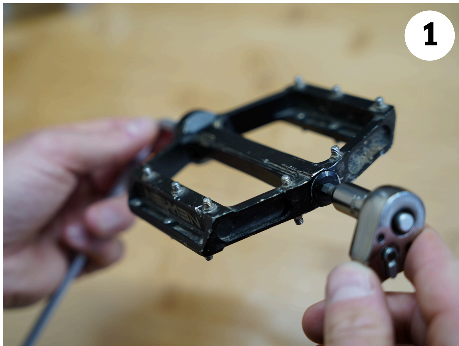
Unscrew the end cap from the pedal with a 5mm hex key.
