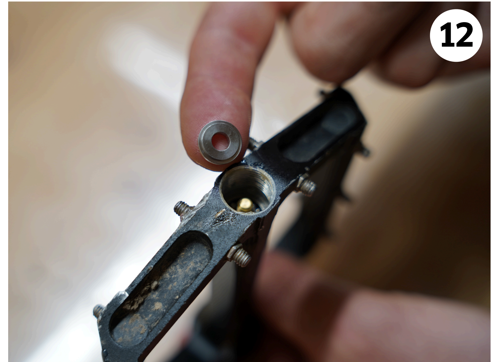
Insert the silver spring washer on the outside of the pedal body.
