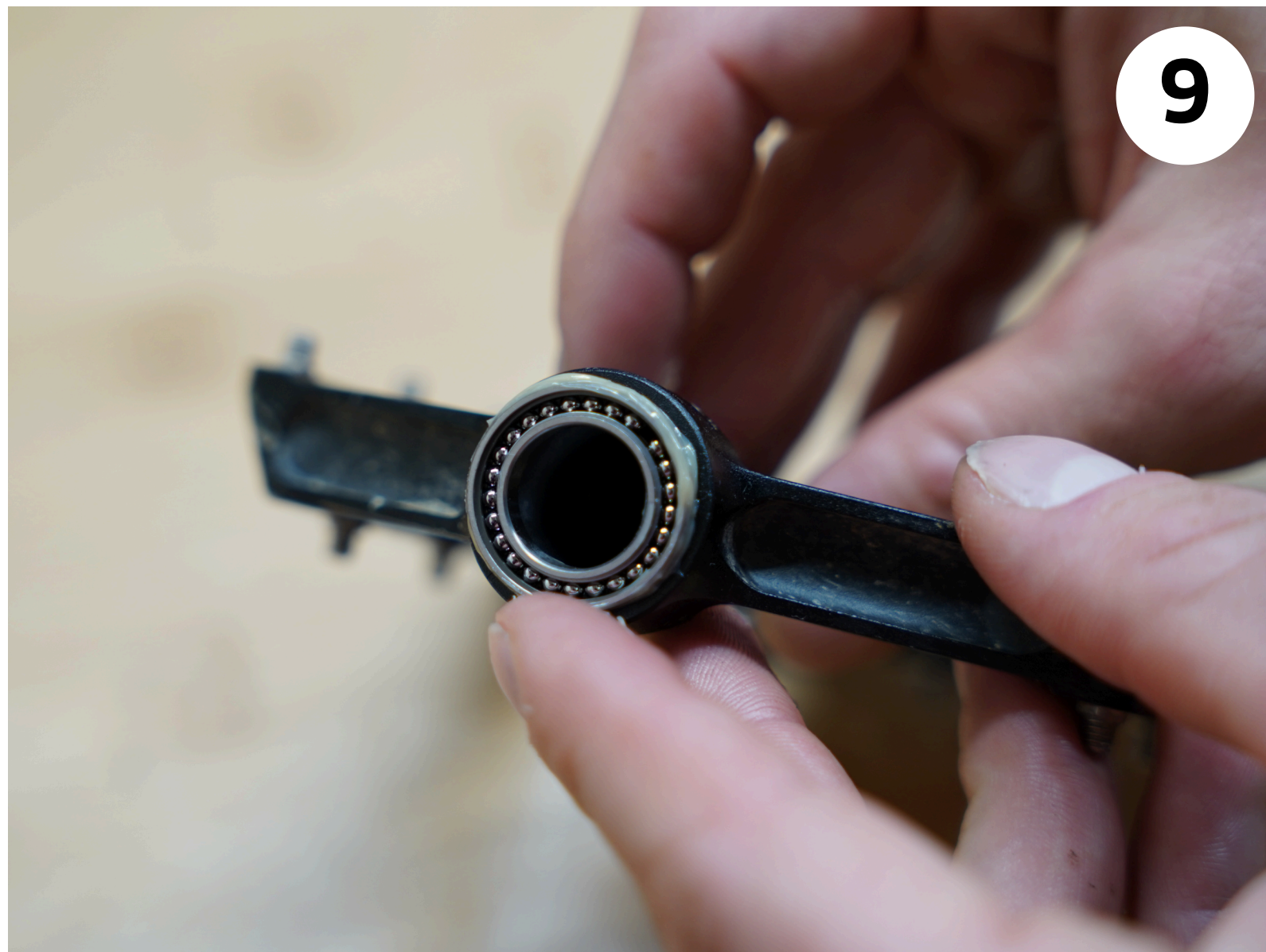
Insert the new bearing on the inside of the pedal body.
