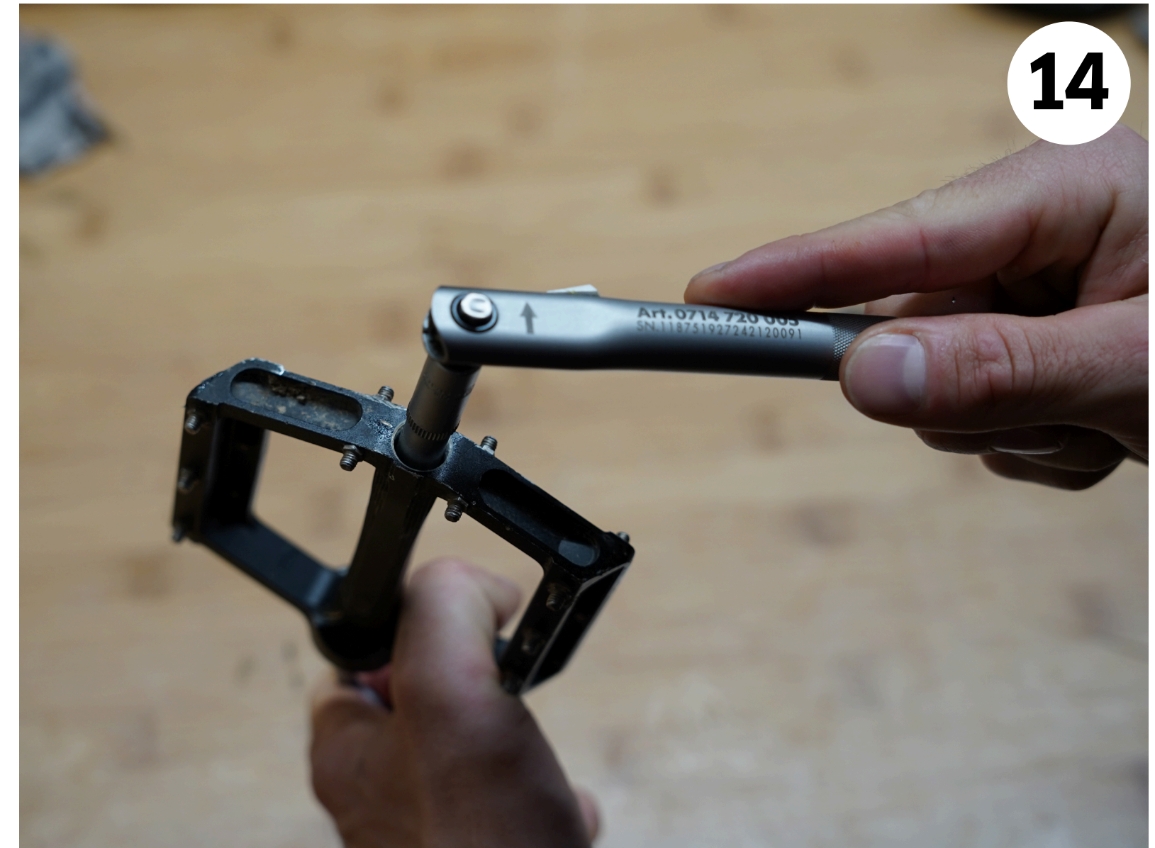
Tighten the pedal M4 nut with a torque wrench to a maximum of 1.5 Nm! Note: The nut for the left-hand side has a right-hand thread, the nut for the right-hand side has a left-hand thread.
