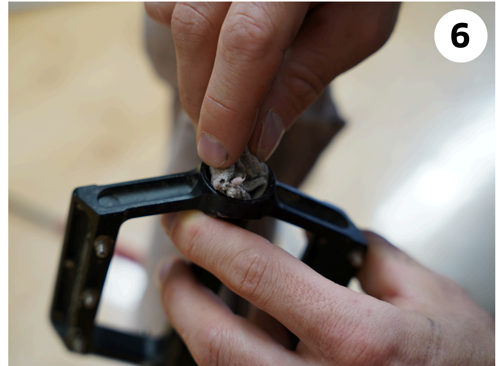
Clean the pedal body and the spring washers and remove old grease.
