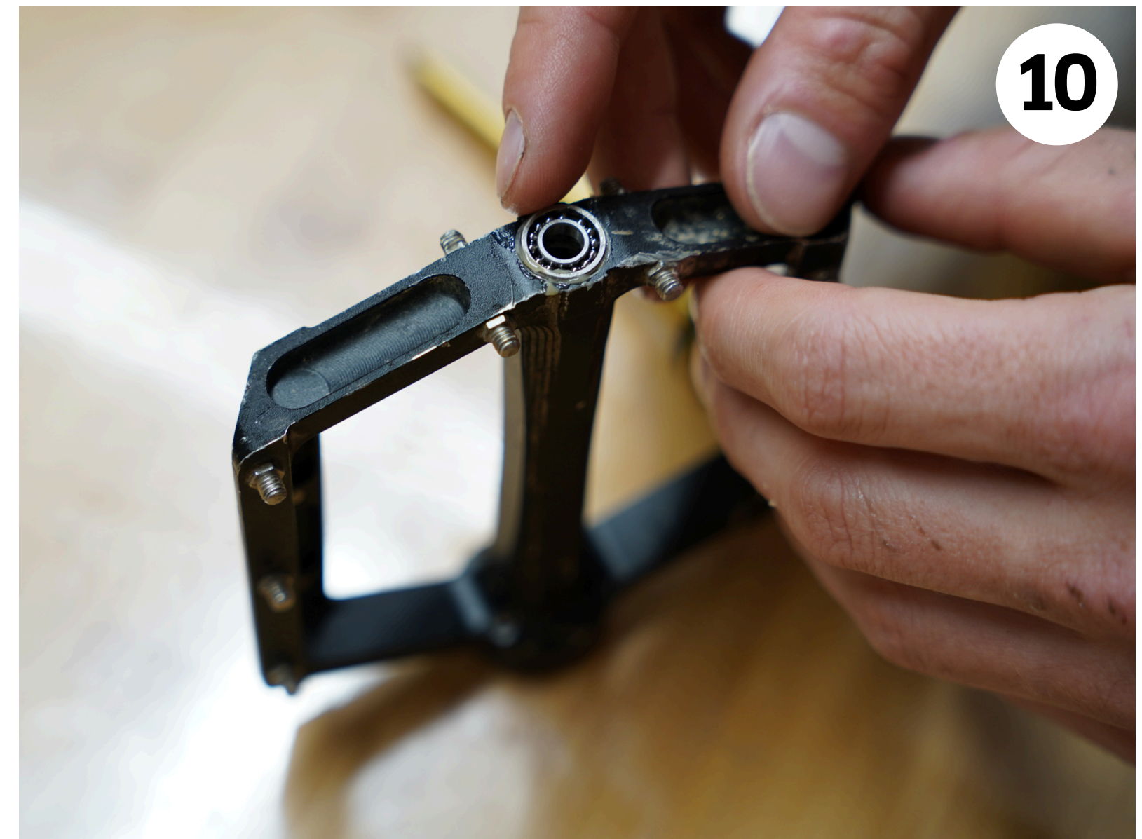
Insert the small bearing on the outside of the pedal body.
