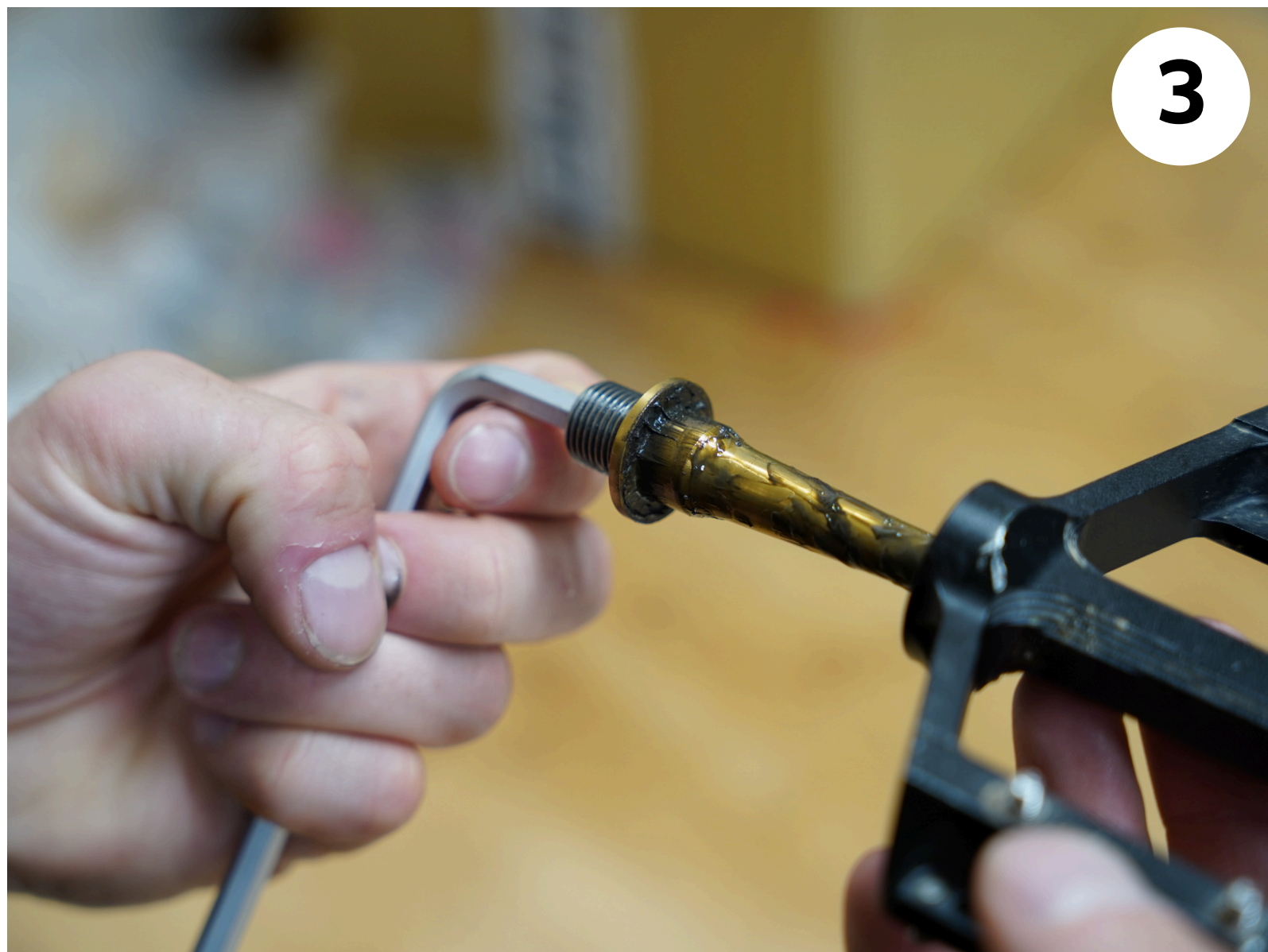
Take the axle out of the pedal body.
