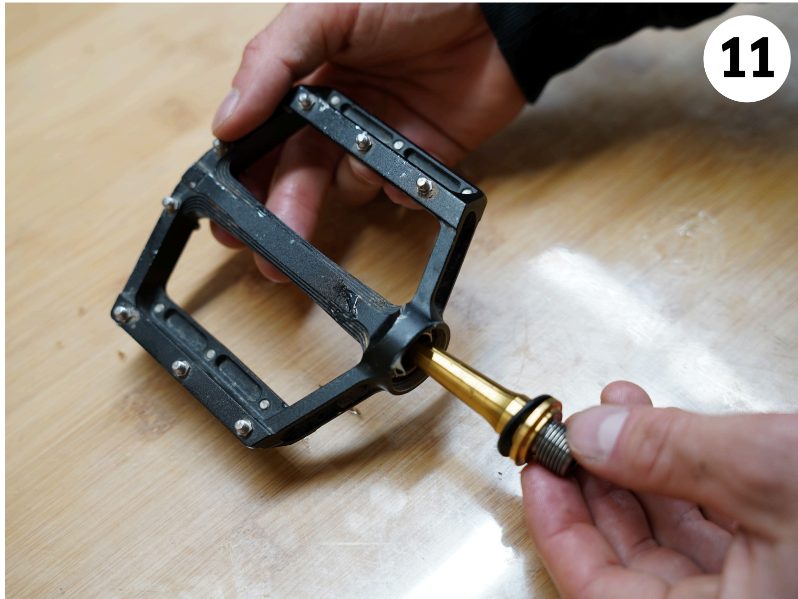
Thread the axle into the pedal body.
