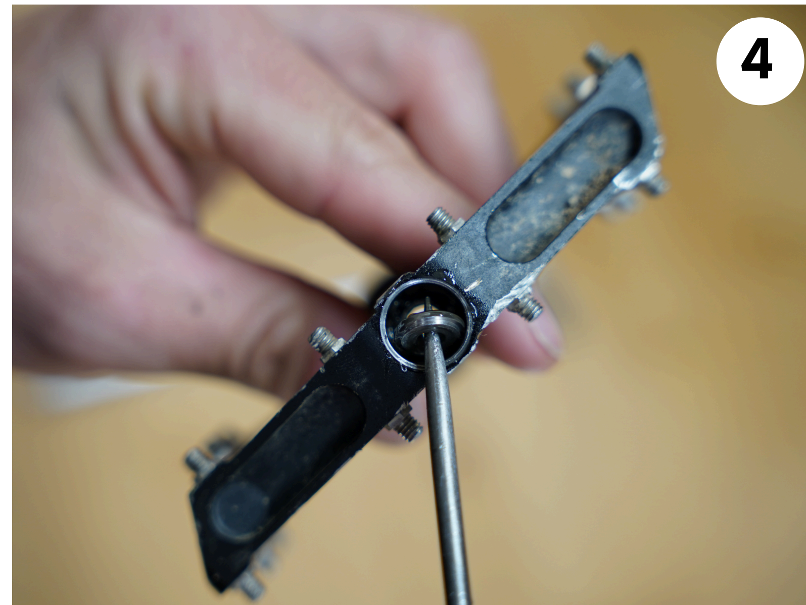
Take the spring washer and the bearing out of the pedal body.
